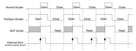
Figure 33. WinX Continuous Cleans Timing Diagram
